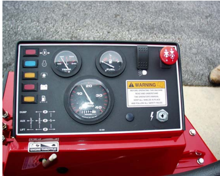
Figure 4.9.b. The key has been removed from the ignition. Untrained operators and little children cannot start the tractor if the key is removed from the ignition.
