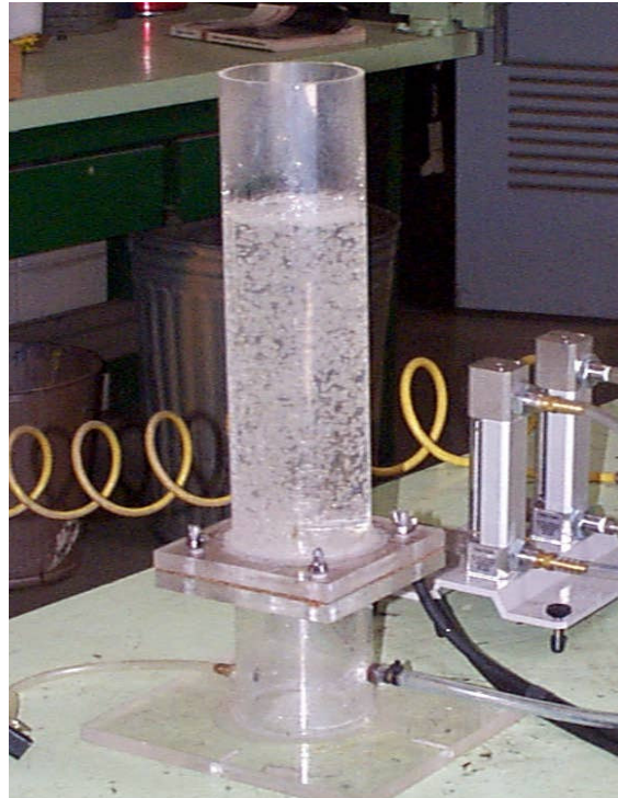
Figure 6: Air bubbling through porous membrane.
